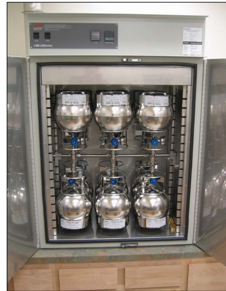
CC-2 12-position Canister Cleaner for 6L Canisters with enclosed oven
