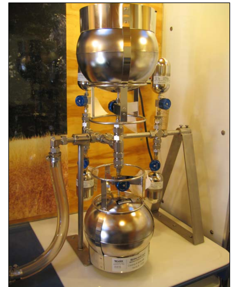
CC-3 6-position Canister Cleaner with 2 each 6L Canisters and 4 each 400ml Minicanisters inside a mobile lab
