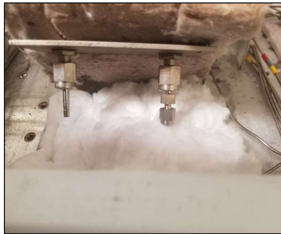
Figure 2. Photo of one approach to disengage Thermal Conductivity Detector from vibrations generated by imbalanced column oven fan motor and transmitted by the instrument chassis. Thermal Conductivity Detector box is tilted back to expose insulation inserted under the detector to effectively suppress the interfering vibrations.
