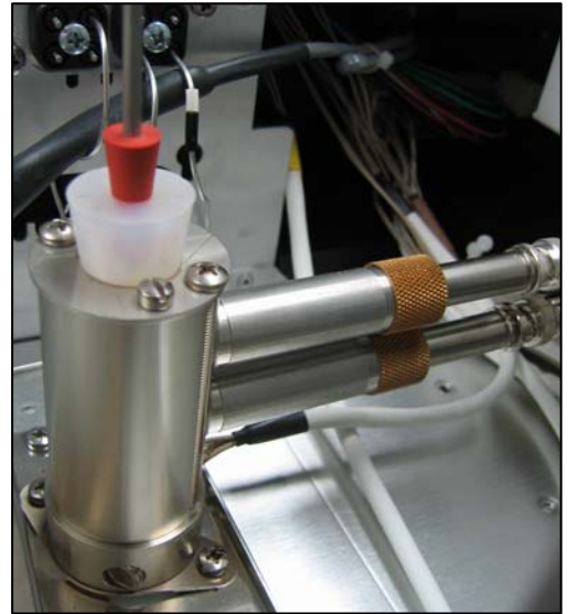
Figure 33. Flows at the detector can be measured by inserting a flow tube and stopper at the top of the detector tower.
