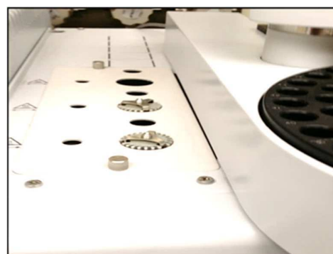
Figure 2. Dual injectors on Scion Gas Chromatographs 1 with Scion 8400 Pro Automated Sampler. 2
