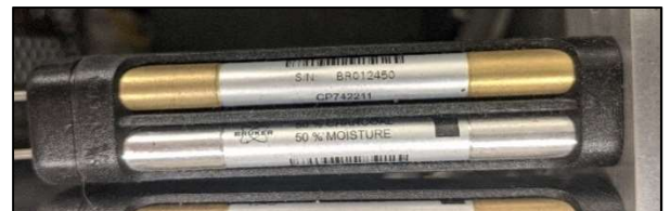
Figure 12. Pencil filters are mounted under the left top cover of the Scion 456 Gas Chromatograph.
