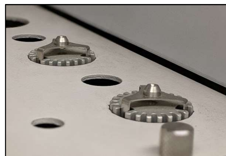
Figure 10. Photo of finned injector nut, with an injector switch to start chromatographic run on injection.
