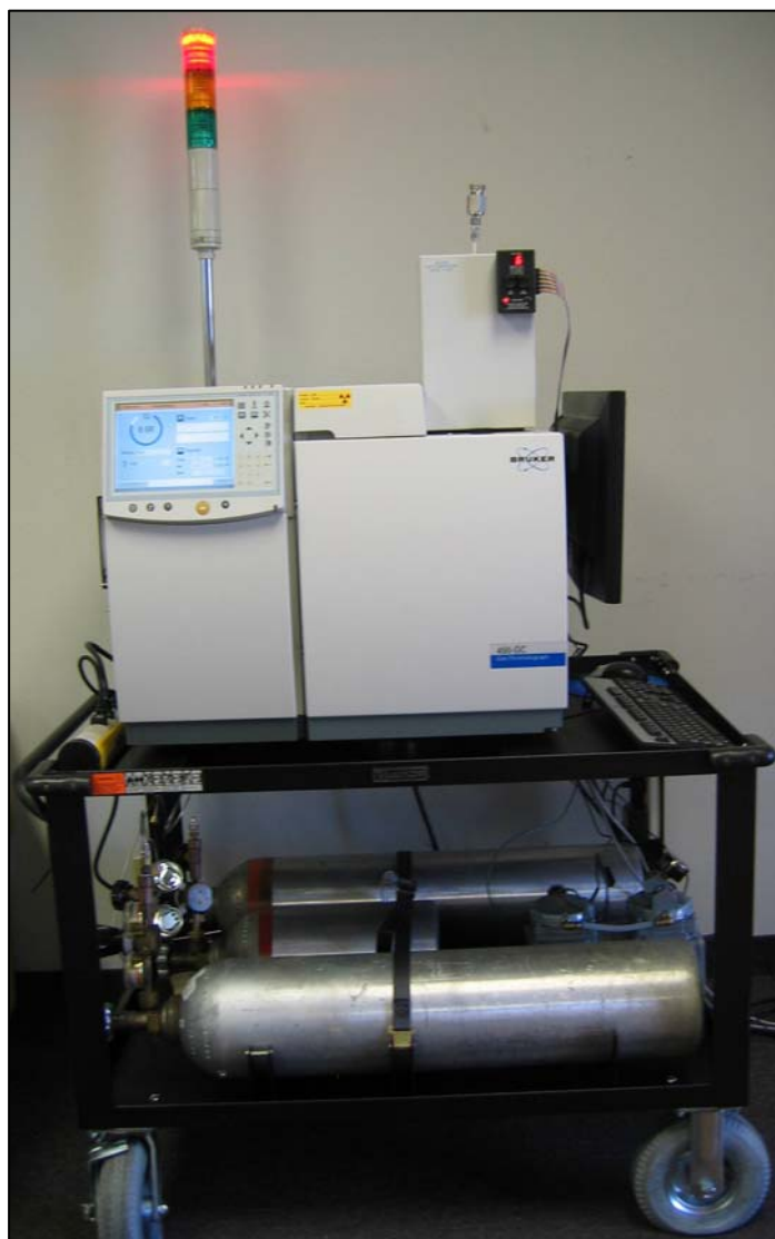
Bruker 450 Gas Chromatograph mounted on a portable cart with supply gases on bottom shelf.
