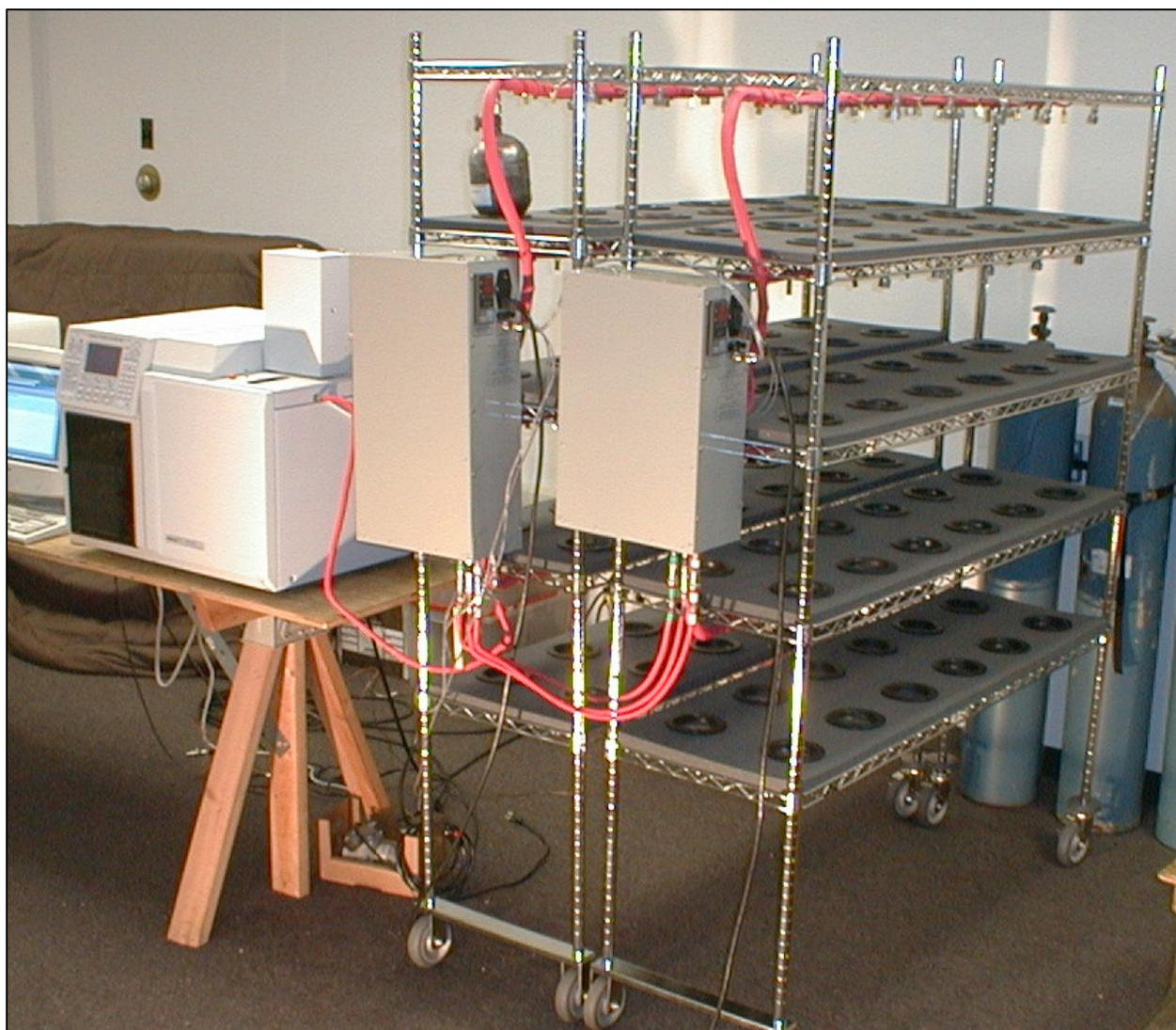
valves. Three electronic flow controllers and two detector electronic flow controllers are included. All seven thermal zones set temperatures for columns, valves, catalysts and detectors. Additional digital flow controllers and pressure regulators provide extra flows. And three external temperature controllers provide for heated sample lines and other thermal zones. The oxidation catalyst is located within its own oven mounted on the instrument's side.
