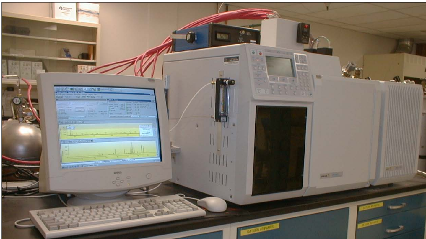
Ultra Trace Toxics System by Lotus Consulting with Varian Saturn 2200 and Sierra Instruments Mass Flow Controller (blue box on top of Varian 3800 Gas Chromatograph).
