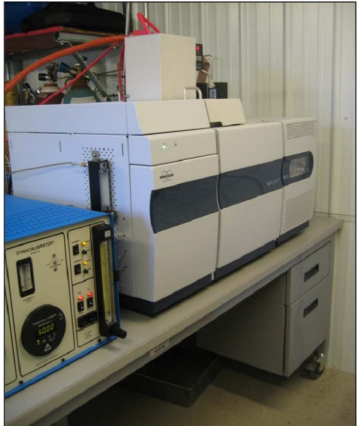
On-Line Toxic Organics/Siloxanes in Biomethane Analyzer at an active landfill.
